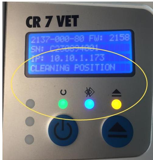
Once the CR7 is in the cleaning position, the front cover needs to come off. You press the silver button in front, then lift the darker grey cover straight up.
